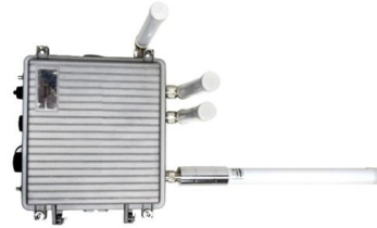
LoRawan outdoor base station
